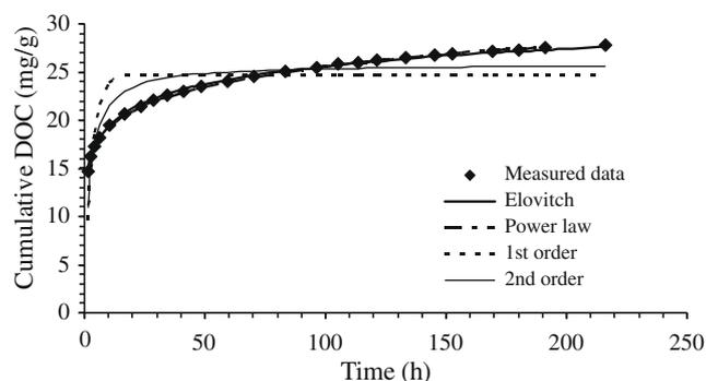
Fig. 2c. Fitted cumulative DOC leached data from measured data and predicted values for hardwood.
