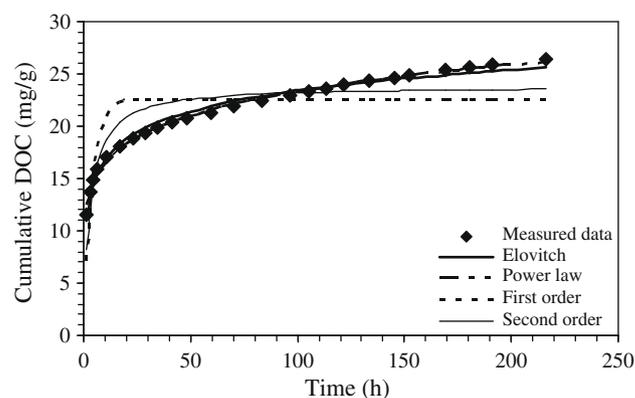
Fig. 2a. Fitted cumulative DOC leached data from measured data and predicted values for compost.
