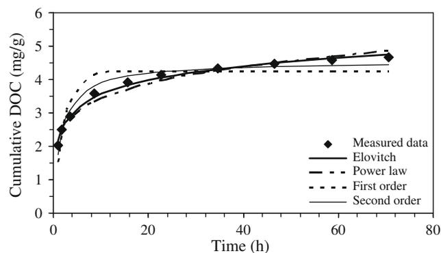
Fig. 2b. Fitted cumulative DOC leached data from measured data and predicted values for pine.
