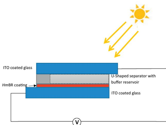
Fig. 7. Schematic structure of home-built photocell, consisting of one ITO with a surface coated with *HmBR* monolayer as working electrode, U-shaped glass separator with buffer reservoir and another blank ITO as a counter electrode.
